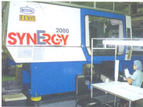
High speed injection moulding machines are installed at CP Packaging's facility for thin wall packaging production
